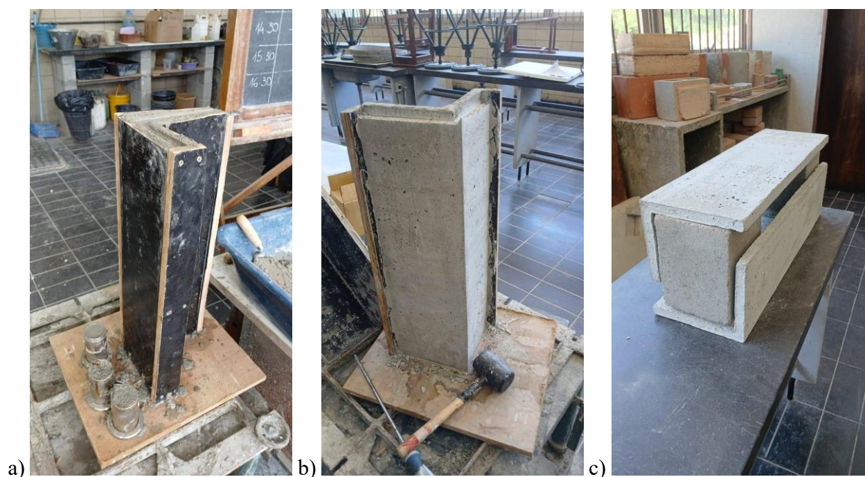
Figure 4: Stages of the construction of the Acoustic Louver A.
